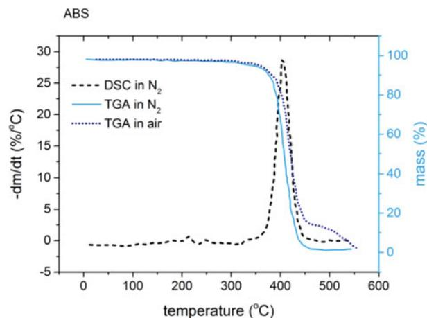
**Figure 1.** DTG and TGA analysis of ASB in N<sub>2</sub> and air atmosphere. Initial mass 0.0484 g.
